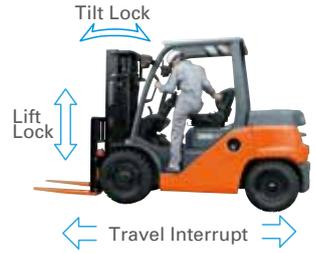
This system uses a switch sensor built into the operator's seat to detect the presence of the operator. If the operator is not in the normal operating position, travel power is interrupted and load handling operations are stopped.
