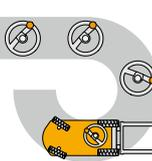
This feature ensures that the angle of the steering wheel corresponds to the angle of the rear steered wheels.
