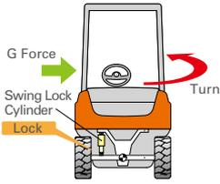
An onboard computer monitors the movement of the forklift and locks the swing of the rear axle when necessary, such as during turns.
