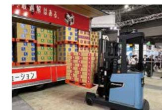
Autonomous lift truck for truck loading and unloading
