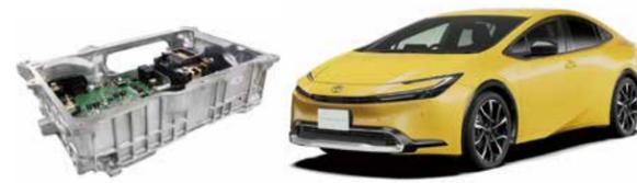
Left: Newly developed compact and high-current DC-DC converter for HEVs
